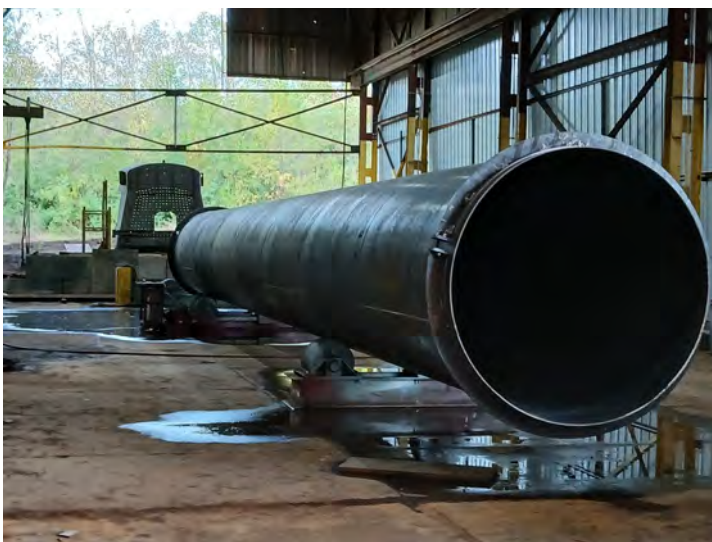
Side view of flare stack
