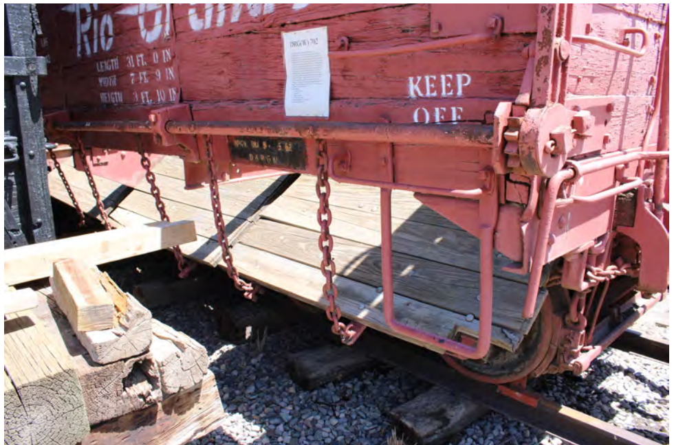
Close-up of the drop bottom doors and mechanism on D&RGW drop-bottom gondola #702 at the Ridgway Railroad Museum in Ridgway, Colorado. The museum obtained the car at a Durango & Silverton silent auction in 2004. Photo by: Jeff Cooper
