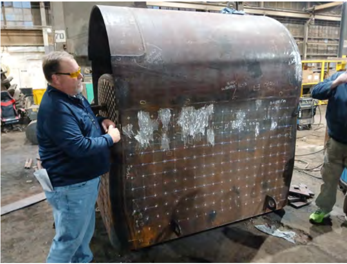
Fred pointing out layout of fire box assembly stay bolts on replacement F&J #112 boiler Shay
