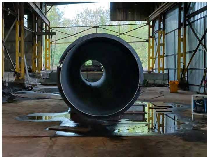
Flare stack, 1st of 3 sections
