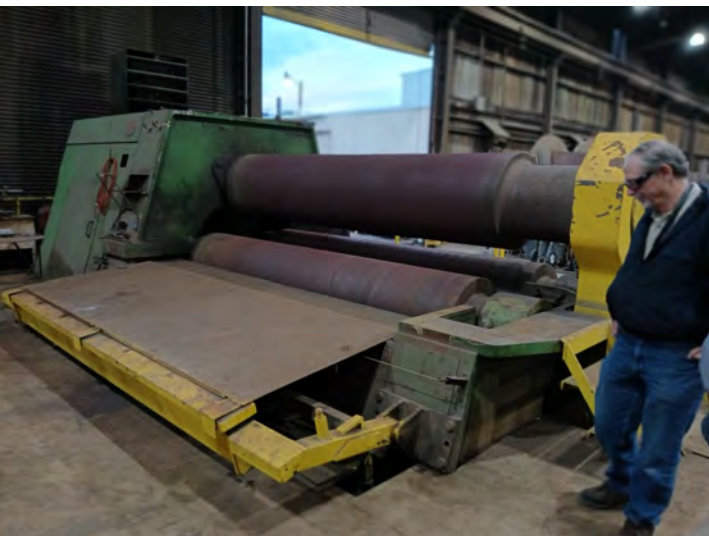
Pyramid roller, will roll up to 6" thick steel plate
