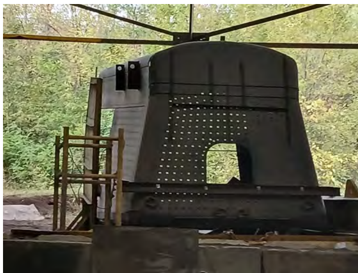
Back of PRR T1 No. 5550, 4-4-4-4, boiler
