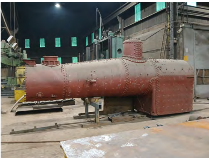
Original boiler, Frost & Johnson Lumber Co., #112, 2-truck, 60 ton Shay
