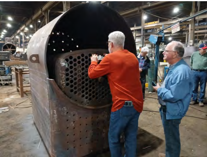
Taking special pictures of fire box assembly
