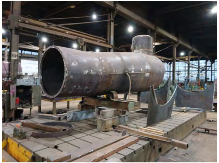
Replacement of original F&J boiler, #112, 2-truck, 60 ton Shay. Created by laser technology
