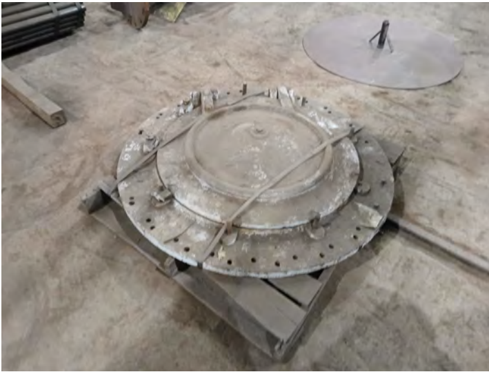
Smoke box door, F&J, #112, 2-truck, 60 ton Shay
