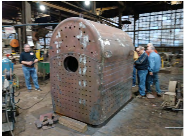
Fire box for replacement F&J, #112, boiler, Shay
