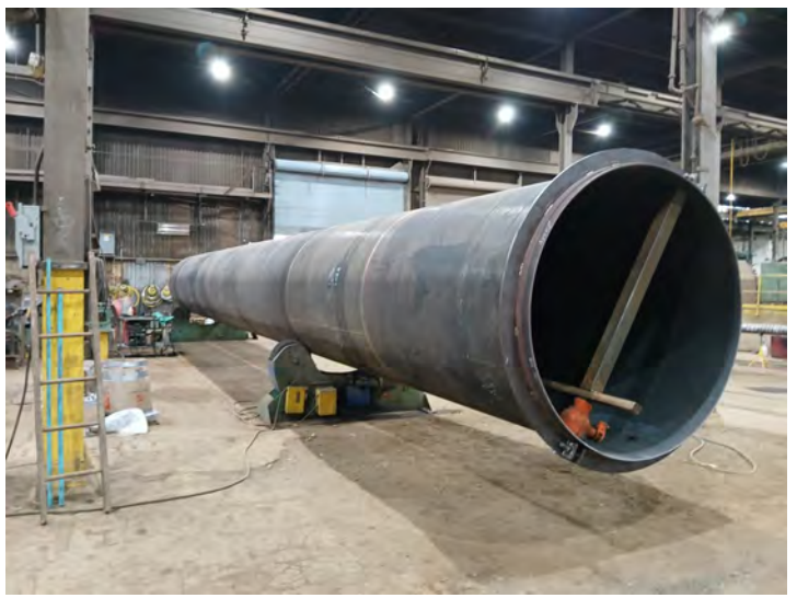
3rd section of flare stack
