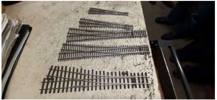
Examples of turnouts made in injection molder press.
