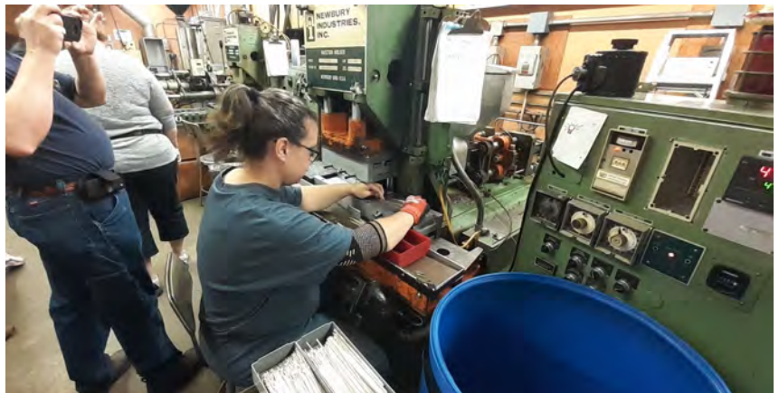
A worker at an injection molder press making a turnout.
