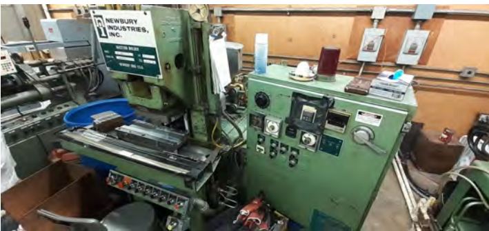
Injection molder press for flex track.
