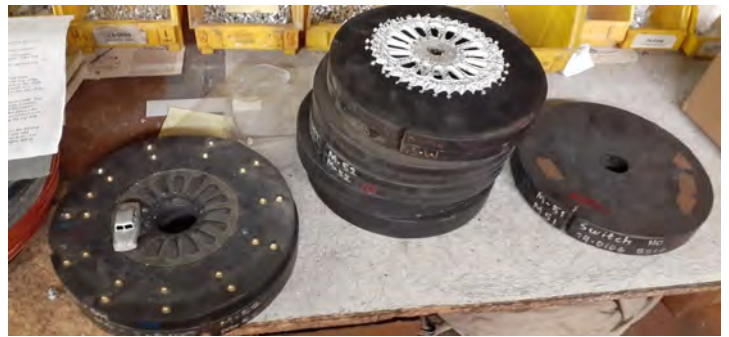
Molds used in the "lost wax casting" process.
