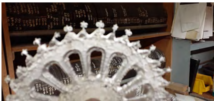
Tiny parts made by "lost wax casting."
